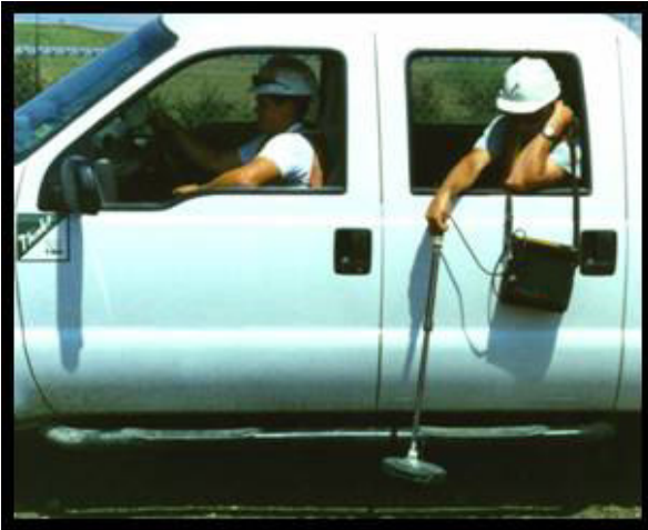
Drive the Duct Path
